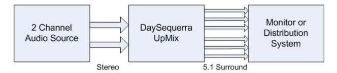
The surround mix produced from the input content is fully immersive to the listener when played through a 5.1 monitor system.
