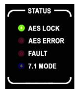
**AES LOCK** - Green LED indicator illuminates when UpMix has acquired a valid AES3 digital input signal.
